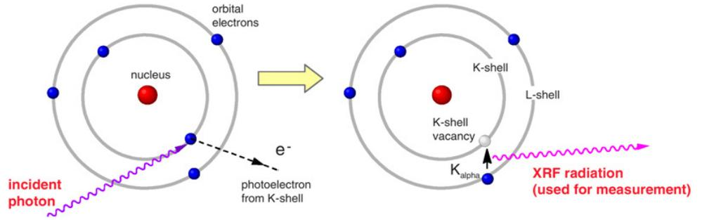
For measurement of thin metallic coatings applied to steel strips this X-Ray Fluorescence (XRF) principle is used: The coated steel strip is exposed to a primary beam of photon radiation. This photon radiation can be gamma rays or X-rays, having sufficiently high energy to stimulate excitation and emission (fluorescence) of X-rays. The excitation of iron atoms in a steel strip leads to emission of fluorescence radiation with an energy of 6.4 keV (1 kilo electronvolt =  $1.6 \cdot 10^{-16}$  J).
