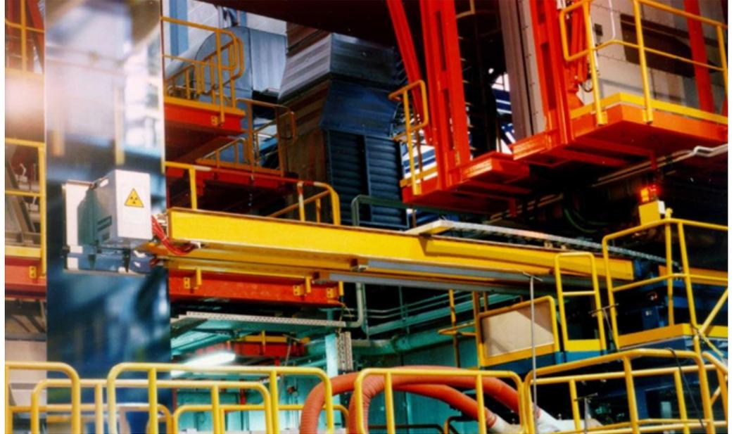
The 'Hot' measuring heads also contain further sensors for measuring the distance from strip to measuring head and temperature. Detector housing and measuring head are water-cooled for use up to 100 °C (373 K) ambient temperature. Additionally the detector windows are cooled by air jets.
