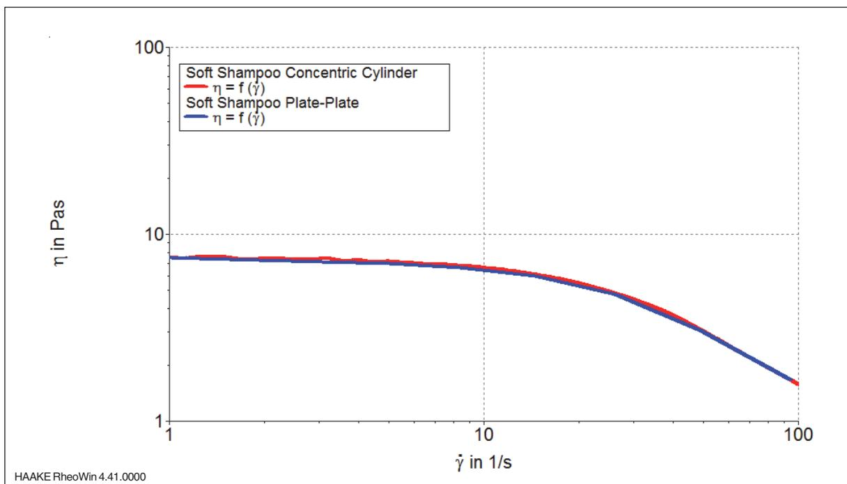
Fig. 4: Viscosity as a function of shear rate for a shampoo measured with concentric cylinders and plate/plate geometry at RT.
