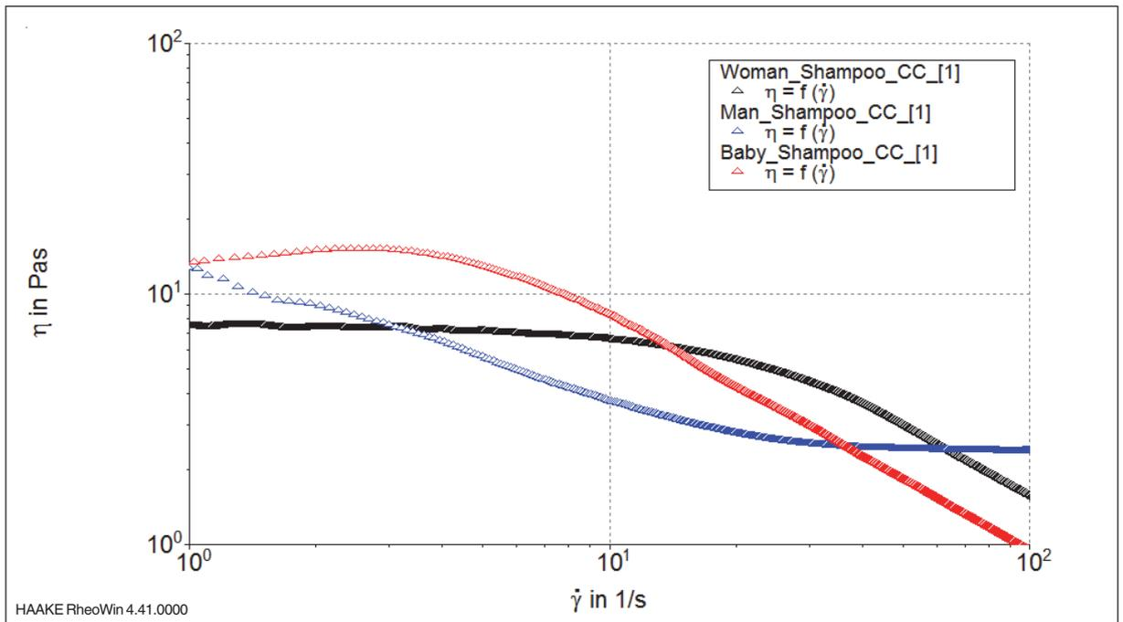
Fig. 3: Viscosity as a function of shear rate for three different shampoos at RT.
