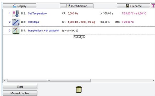
Fig. 2: HAAKE RheoWin Measuring Routine to determine the viscosity as a function of shear rate on the Thermo Scientific HAAKE Viscotester iQ
