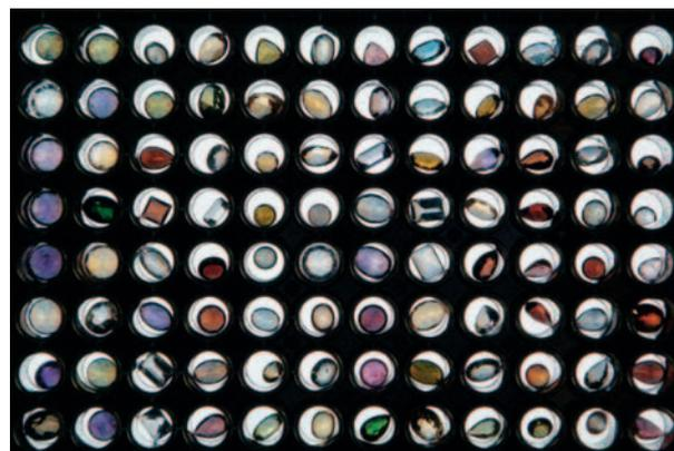
Figure 2: The glass bottomed 96 well plate loaded with semiprecious gemstones
