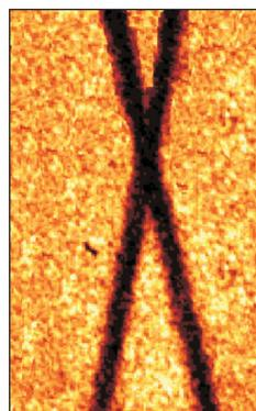
Figure 3: C 1s image of the PET substrate. Image collected in 5 minutes.
