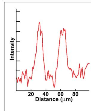
Figure 2: A line scan extracted from the C 1s image of the fiber, showing that the spatial resolution in the image is better than 2  $\mu\text{m}$ .
