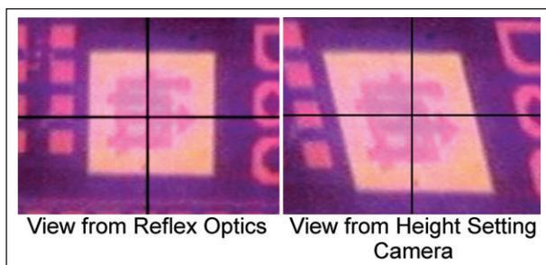
Figure 7: Views of the sample in the analysis position. The same feature is centered in each view and so the sample is at the correct height.
