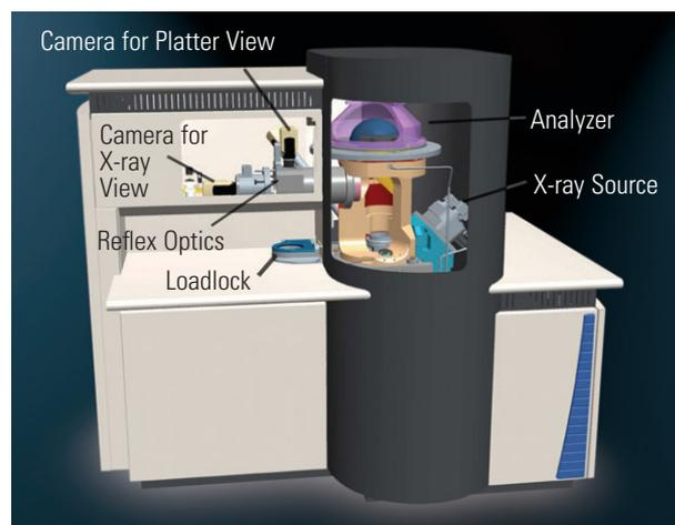
Figure 2: Some of the component parts of K-Alpha
