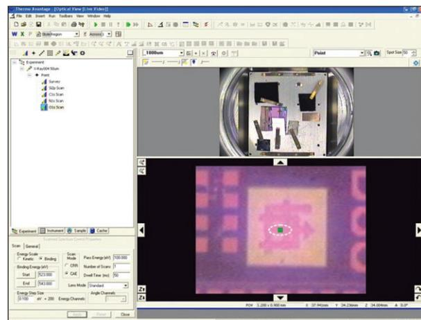
Figure 6: Screen shot from the Avantage data system showing two optical views. The upper image is the Platter View, recorded at sample entry, showing all of the samples loaded onto the sample holder. The lower image is the live Reflex View of the analysis position. In each case the analysis position is clearly marked. Both views are always available to the analyst.
