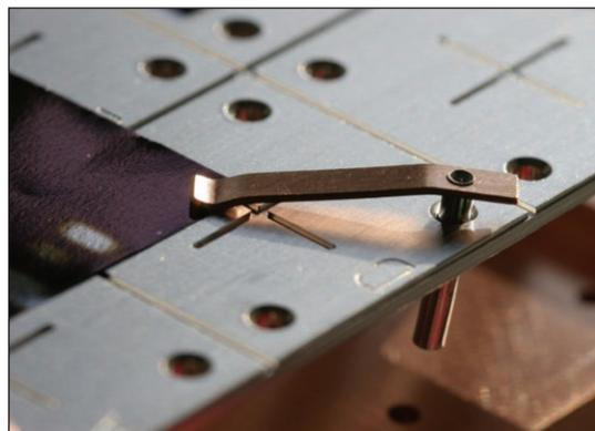
Figure 5: Sample clipped in place on K-Alpha sample holder
