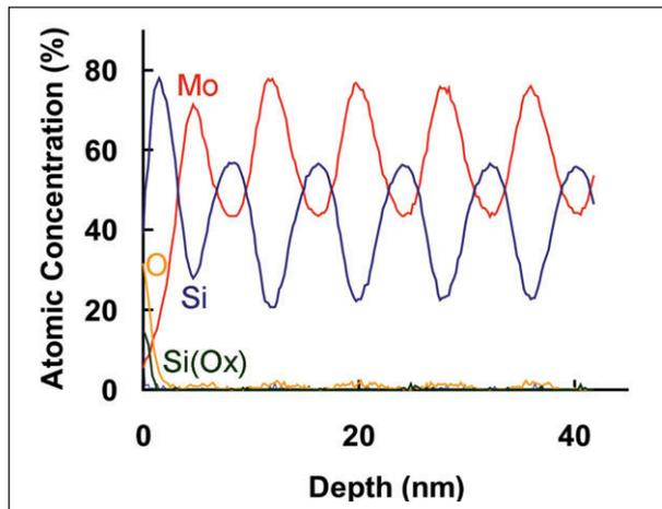
Figure 11: Depth profile of an X-ray mirror having 7 nm repeats. The argon ion energy used for this profile was 200 eV.
