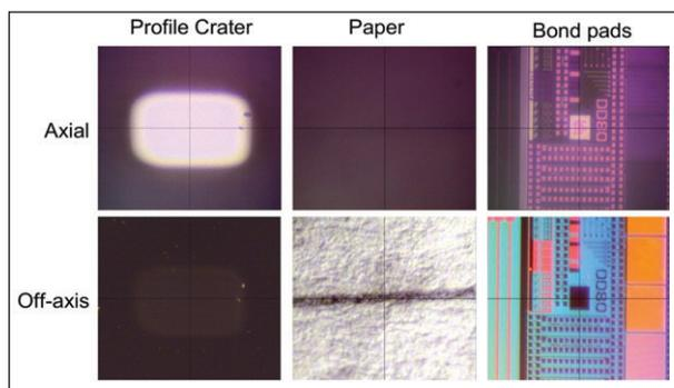
Figure 8: Three sample types each illuminated by axial and co-axial lighting
