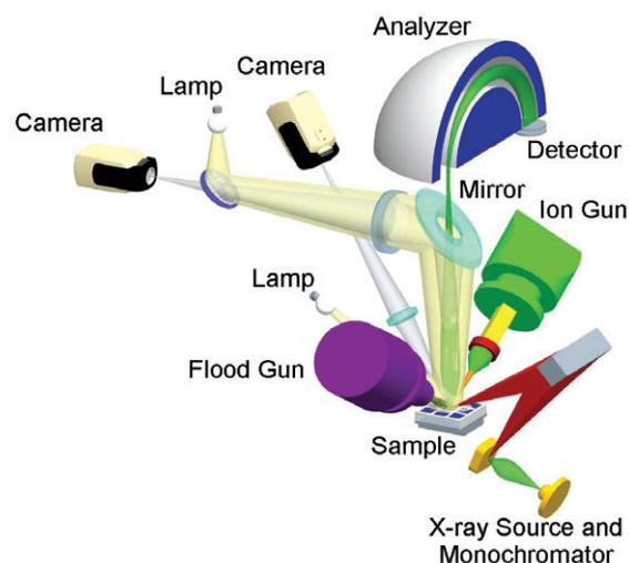
Figure 3: The internal geometry of the analytical components in K-Alpha
