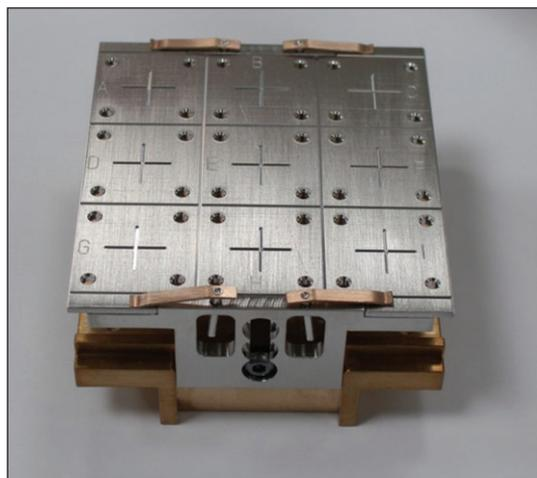
Figure 4: The sample holder for K-Alpha.
