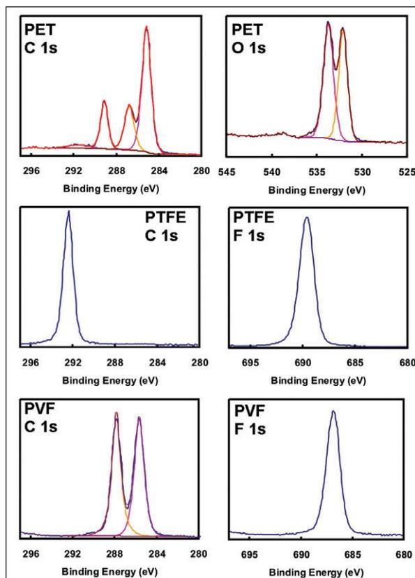
Figure 9: C 1s spectra from a series of polymer surfaces
