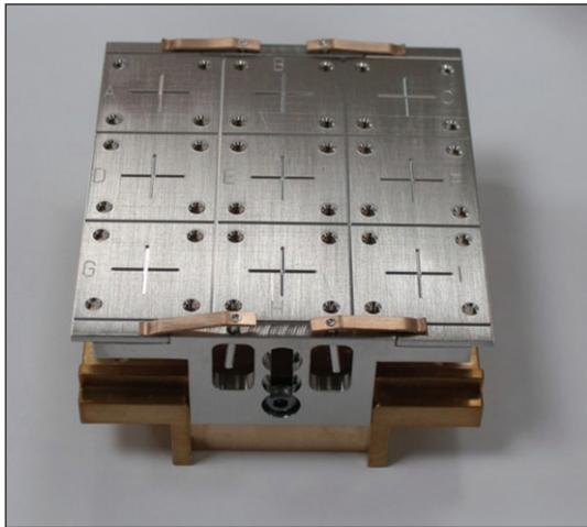
Figure 4: The sample holder for K-Alpha.
