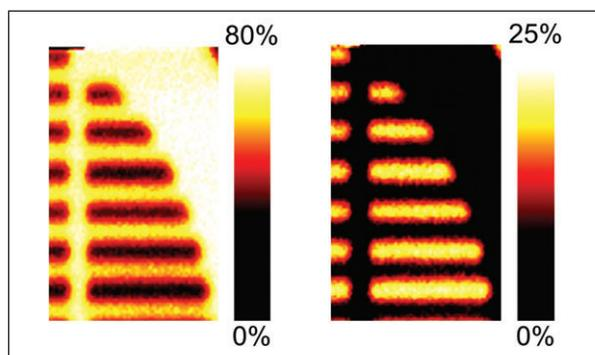
Figure 10: (a) Atomic concentration map from the hydrocarbon peak following peak fitting at every pixel. (b) Atomic concentration map from the fluorocarbon peak.
