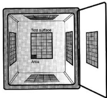
**Figure 1:** Incubator sample chamber and glass door. Distribution of the test surfaces and individual areas for artificial contamination with various germ species
