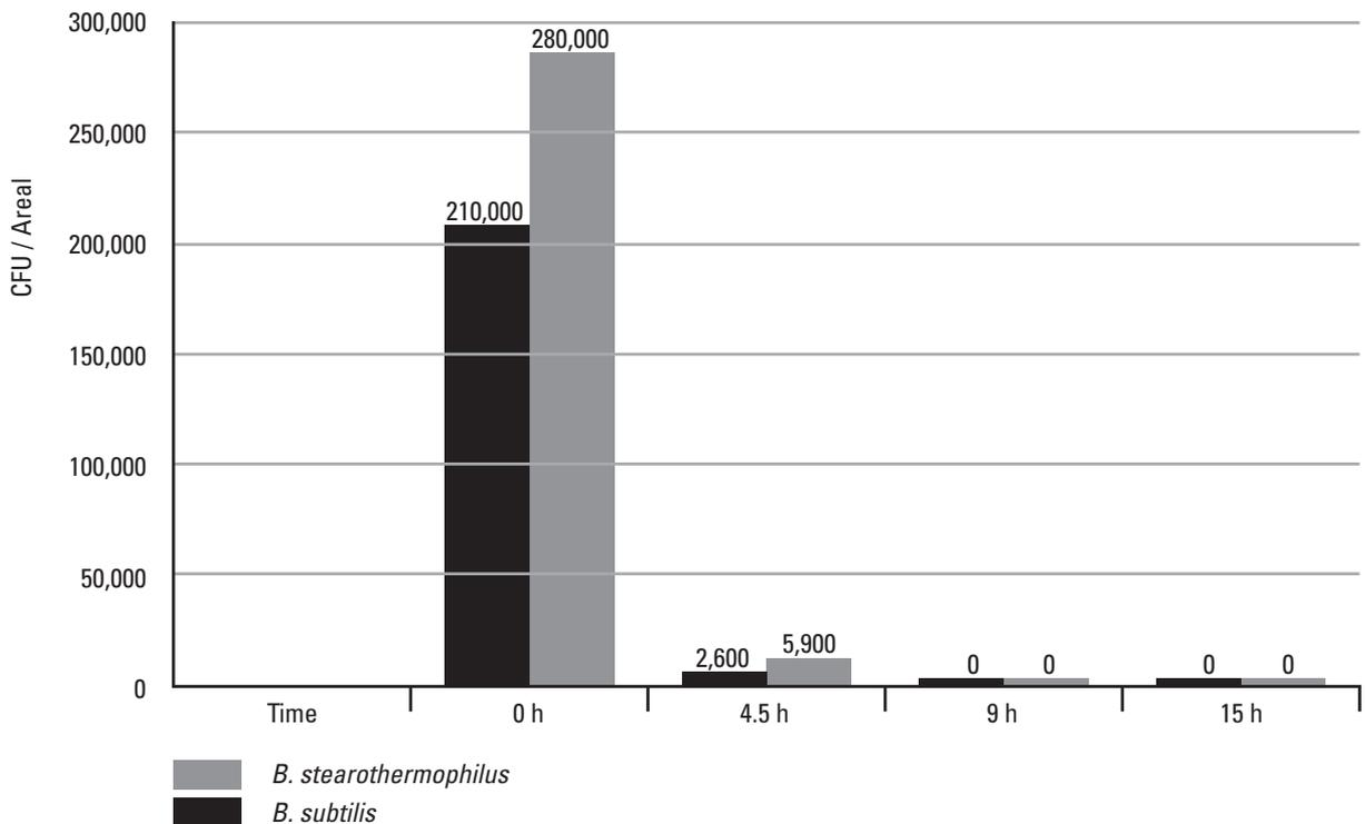
Figure 2: Time dependent kinetics of germ reduction. Bacillus spores at 90°C and moist heat.
